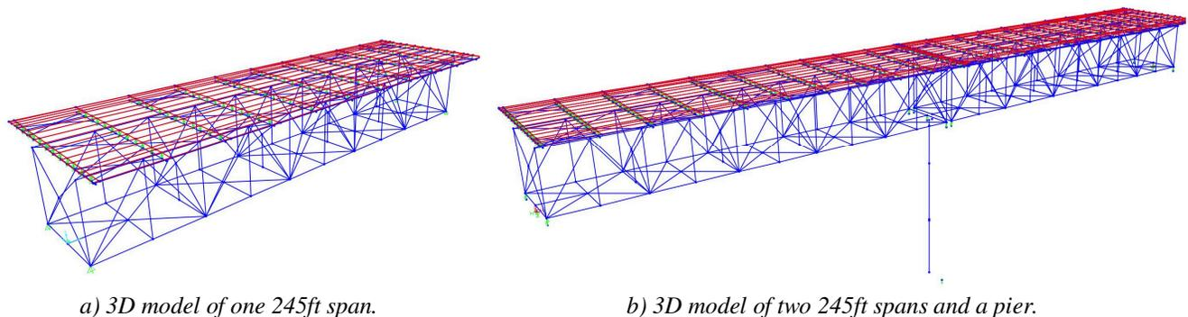
a) 3D model of one 245ft span.
