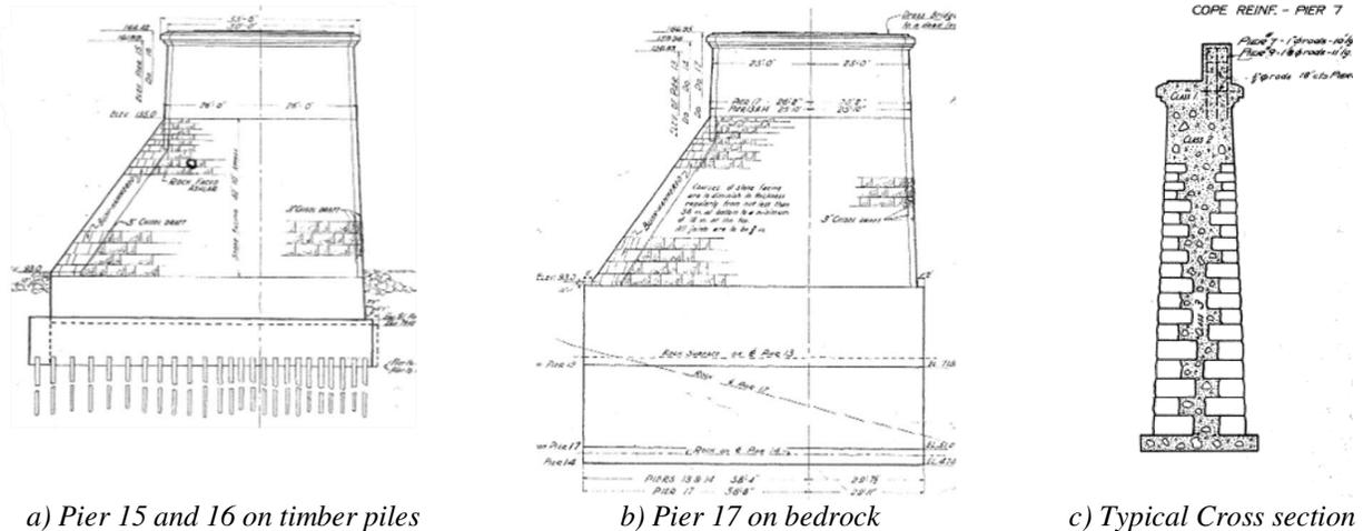
Figure 6. Details of typical south approach piers.
