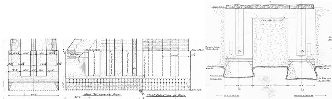
Figure 5. Foundations for Piers 24 (left) and 25 (right).
