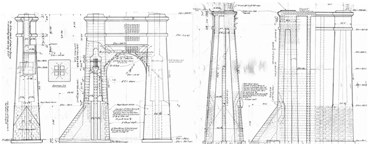
Figure 4. Piers 23 (left, 26 similar) and 24 (right, 25 similar) elevations showing hollow section.
