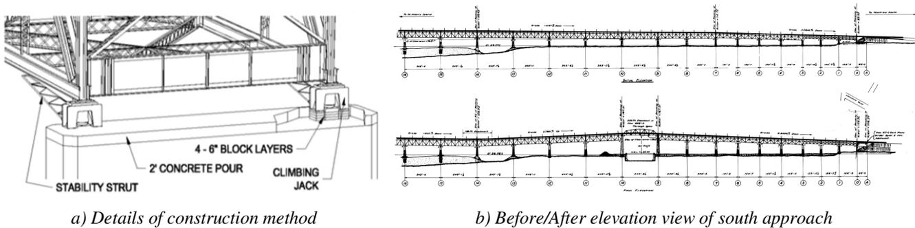
Figure 7. Modifications to the south approach for construction of the Seaway channel.
